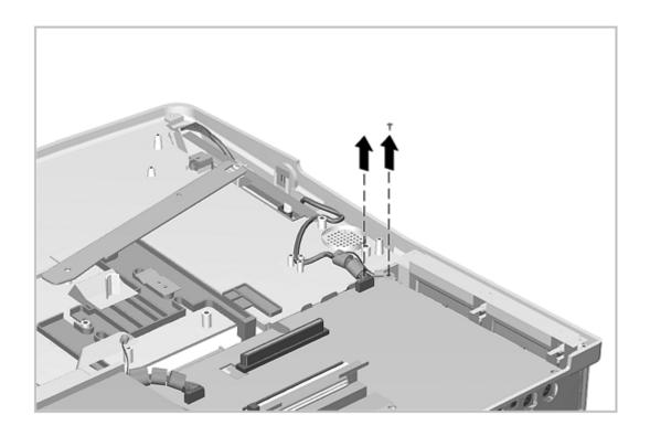
Figure 7-27. Disconnecting the Power Switch Board
